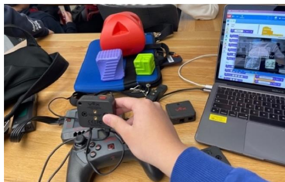
Fig. 2: The vision sensor in action (with vision utility on, detecting the color signatures of the game elements for VIQRC Full Volume)
