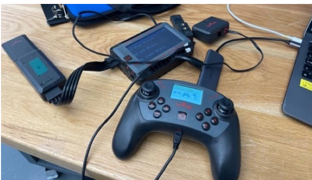
Fig. 1: (messy) Layout for testing the vision sensor. The program running is the example code in VEXcode entitled "Detecting Objects (Vision)"
