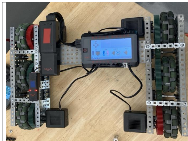
Fig. 1: Drive Train with stiffeners added on
